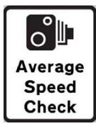
In working with Highways England and their assigned Contractors Average Speed Detection Systems are installed at road works on the Motorway Networks. Their primary function is to protect the safety of the work force through bringing about a greater compliance to the temporary speed limit, which is often set at 50mph.
